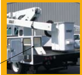
Rear access doors for storage of long fluorescent tubes
