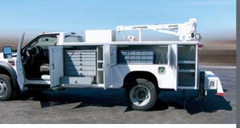
**LIFTMOORE MODEL 3200REE-15** heavy duty corner mount electric crane, installed at curbside rear on top of body, with boom stowed to the front over curbside compartments.
